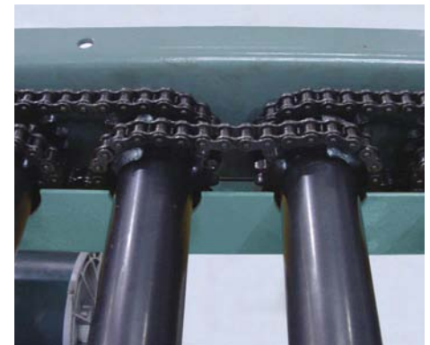
Chain guard removed to illustrate roll-to-roll drive chain. WARNING: Do not operate conveyor with chain guard removed.
